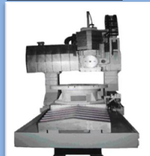
FAMS: A Five Axis CNC Machining System for High Precision Milling and Grinding of Silicon Carbide Satellite Mirrors
